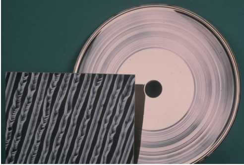
Magnified surface of a typical stereo recording produced on a 305mm (12 inch) p.v.c. disc
